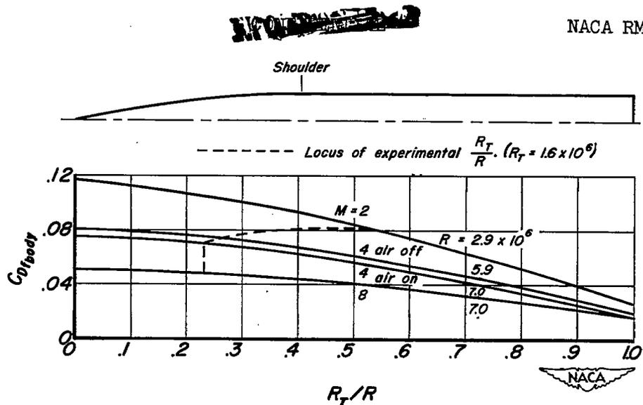
Figure 7. - Variation of theoretical body-alone friction drag coefficient with location of boundary-layer transition.
